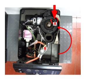
Caution in the new coffee grinder with the screw, Unscrew this last, before disassembly of the upper coffee grinder support.
