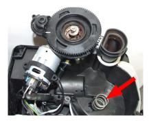
When reassembling the coffee grinder, make sure the spring is repositioned correctly (see photo).
