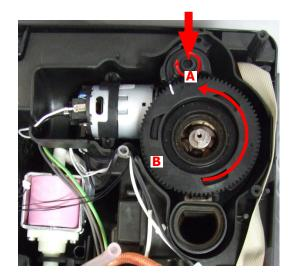
To extract the top support of the appliance, press on the grinding adjustment spindle (A) and turn the support anticlockwise until it unhooks.
