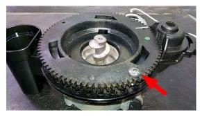
The new machines have a coffee grinder with the screw to prevent the disassembly of the upper coffee grinder support (see photo).
